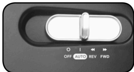
▲ Power switch in auto position
